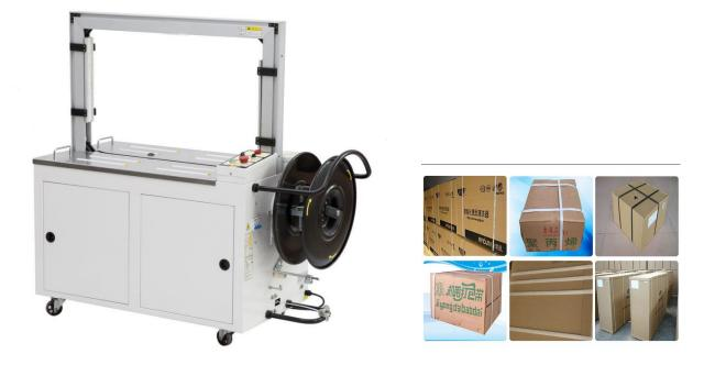
The automatic strapping machine uses a strap to bind the product or package, then tighten it and combine the two ends with a heating iron. The function of the strapping machine is to reinforce the packaged goods, so that the goods will not be scattered due to inadequate tying during handling and storage, and at the same time they should be tied neatly and beautifully.
