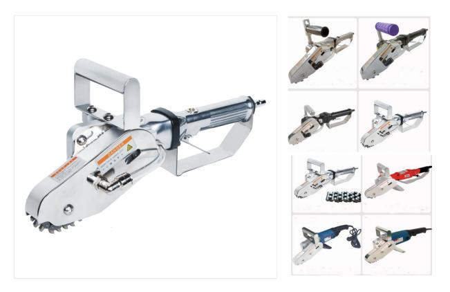
The waste stripper is a high-speed cycle operation driven by the air motor to drive the toothed chain, using sharp teeth to pull out the waste paper edge. It is a pneumatic tool used for the waste removal of cardboard, fine corrugated and ordinary corrugated paper in the printing industry. It can replace the manual hammer to remove waste, improve work efficiency and shorten the waste removal cycle.
