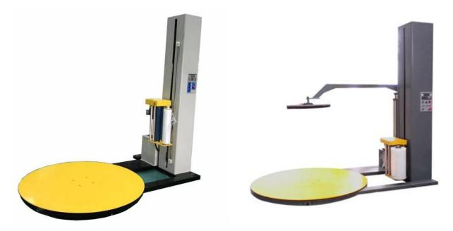
Pallet wrapping machine uses LLDPE stretch film to wrap bulk pallet goods. It is widely used in glass products, hardware tools, electronic appliances, paper making, ceramics, chemicals, food, beverages, building materials and other industries. This equipment can improve logistics efficiency and reduce the loss during transportation. It has the advantages of dust-proof, moisture-proof, and reduced packaging cost.
