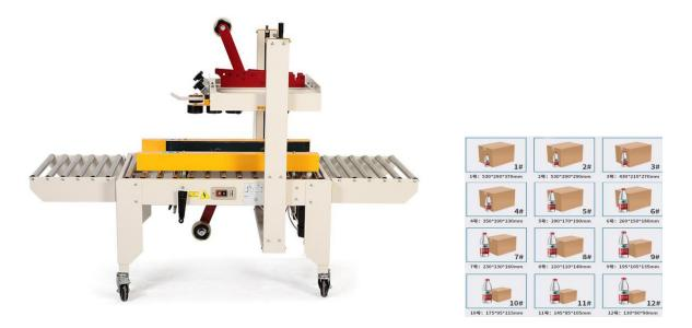
Carton sealing machine is a commonly used packaging machine. It uses BOPP adhesive tape (also called carton sealing tape) to seal the carton. The upper and lower sides of the carton can be sealed at the same time. It has features of fast packaging speed, light weight and durability, simple operation, labor saving and high efficiency. This machine can be used as a stand-alone machine, or it can be used in conjunction with an assembly line.
