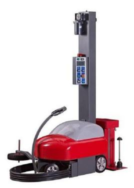
Robot wrapping machine uses LLDPE stretch film as packaging materials and is applied to pallet packaging. It is mainly aimed at a self-moving wrapping packaging machine designed for the user's packaging that is relatively large and heavy and inconvenient to move. the machine can move by itself while realizing the wrapping of the objects. it is simple to operate and has a low failure rate. it is a user ideal choice.
