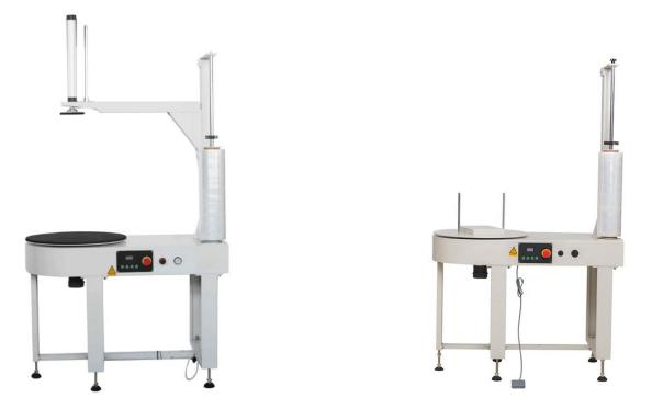
The min stretch wrapping machine uses PE wrapping film to wrap the bulk pallet goods. This model is suitable for small and light goods. It is widely used in glass products, hardware tools, electronic appliances, paper-making, ceramics, chemicals, food, beverages, building materials and other industries.
